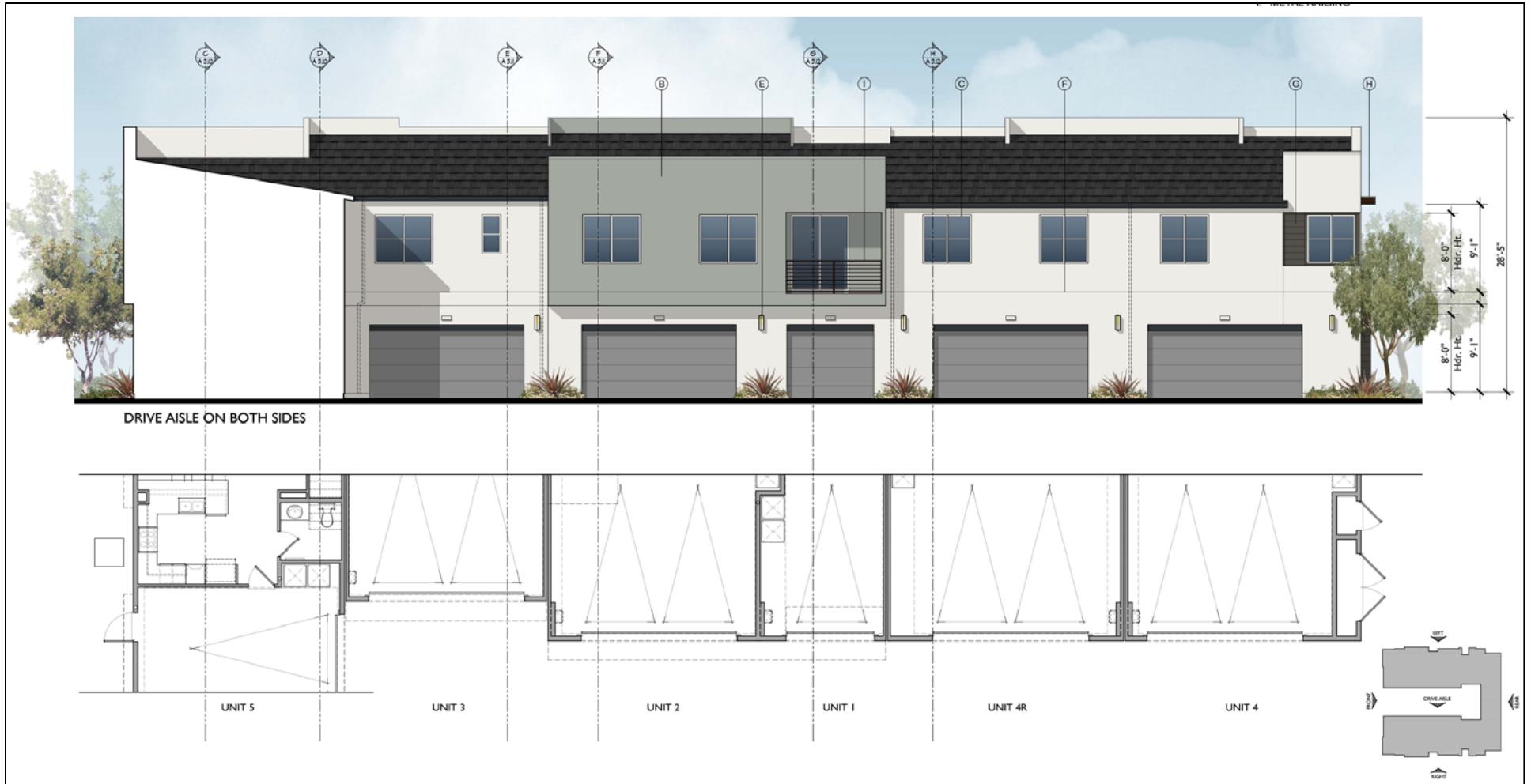
Interior Drive Aisle Elevations
