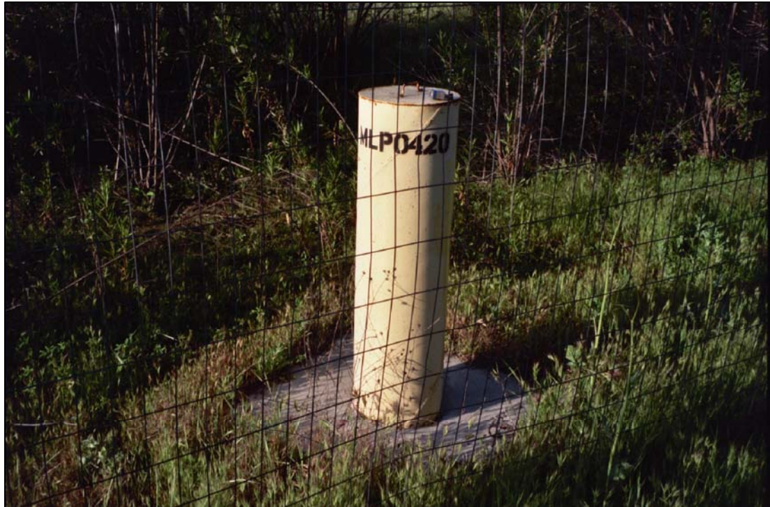
LOOKING SOUTHWEST AT A PERIMETER PROBE FOR MONITORING LANDFILL GAS NEAR THE NORTHWEST CORNER OF THE MILLIKEN SANITARY LANDFILL.
