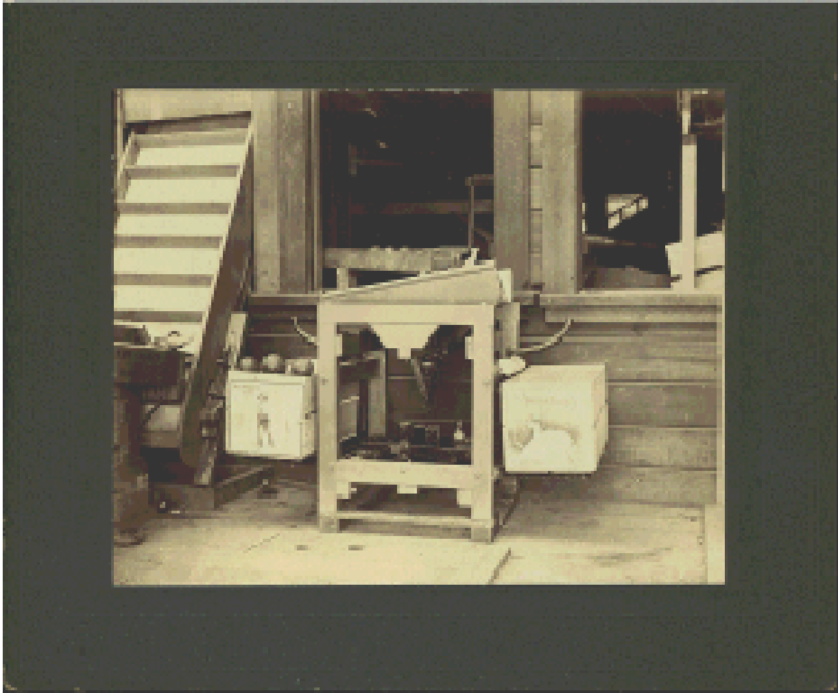
Photo: 1890s automatic orange weighing machine designed and constructed for Redlands Citrus Association. (courtesy of the Ontario Public Library, Model Colony Room, Ontario, CA)
