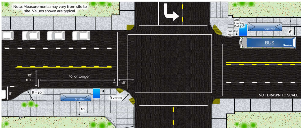
Figure 5-8: Extended curb installed at intersection.
