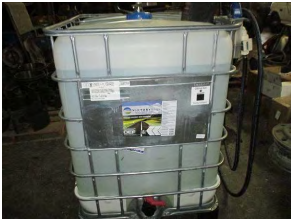
Photo #17 View of the 275-gallon tote of diesel exhaust fluid located in the truck repair shop.
