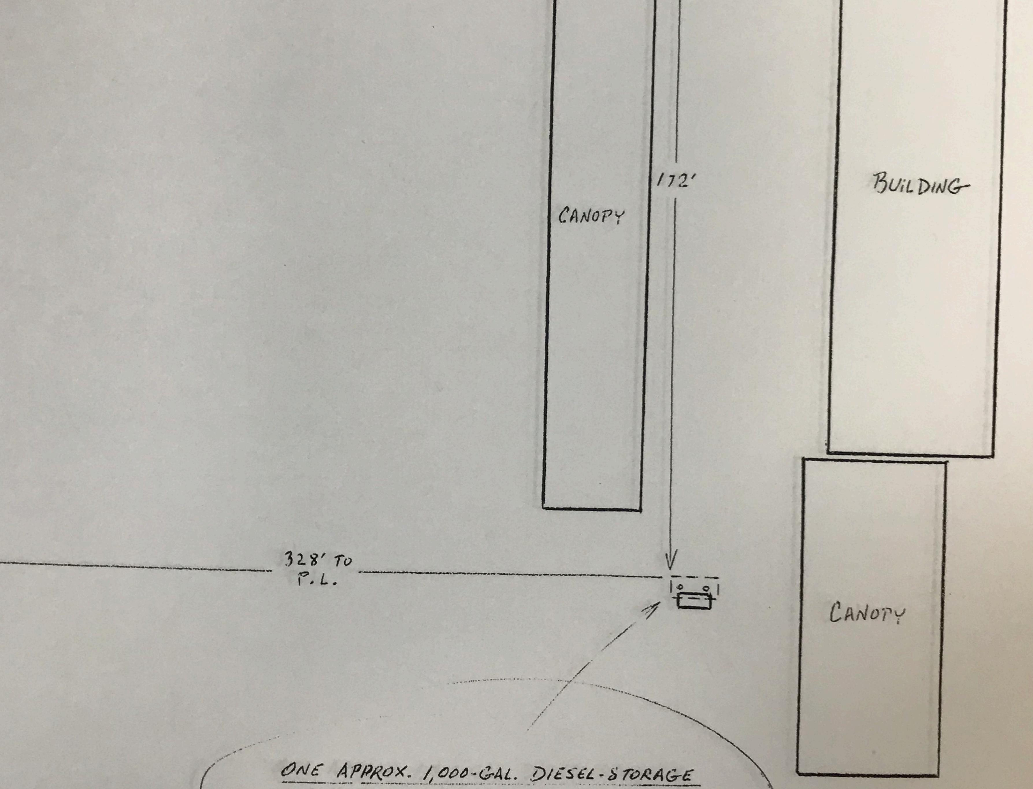
UNDERGROUND STEEL TANK AND RELATED PIPING AND DISPENSER ISLAND TO BE REMOVED.
