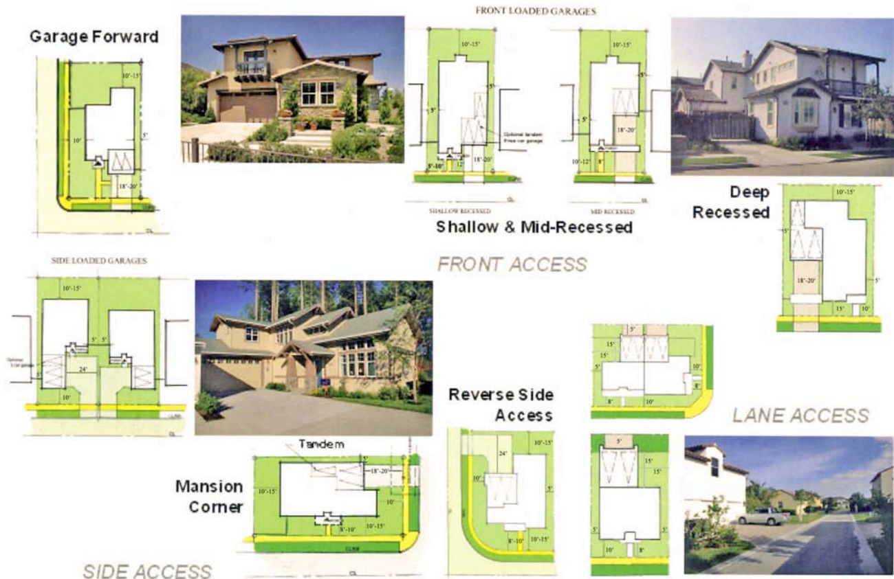
EXHIBIT 8-12: GARAGE PLACEMENT ALTERNATIVES
