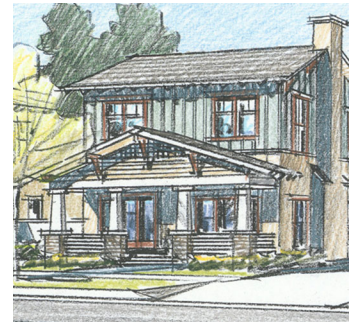
Covered porch with paneled wood siding and wood trims.
