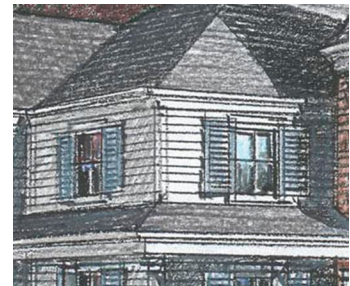
Multi-paned windows with shutters and lap siding.
