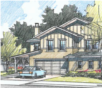
Pale tones with bright white trim, use of stucco and board and batten siding break up two story massing.
