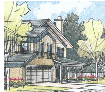
Simple post and beam support at porch.
