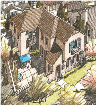
Siding accent at gable end, use of pot shelves and Juliet balconies to activate the street scene.
