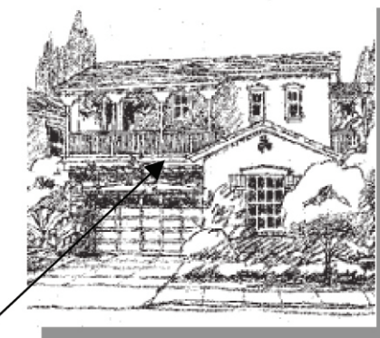
Cantilevered Second Floor Porch
