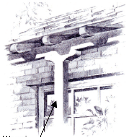
Corbeled Wood Columns
