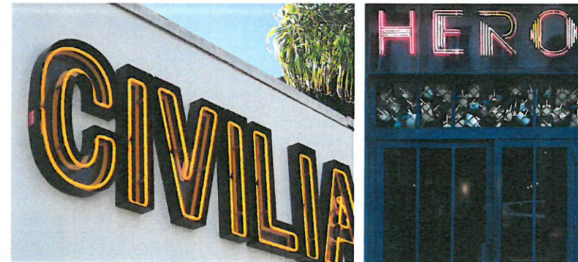
INDIVIDUAL LETTERS WITH EXPOSED LIGHTING
