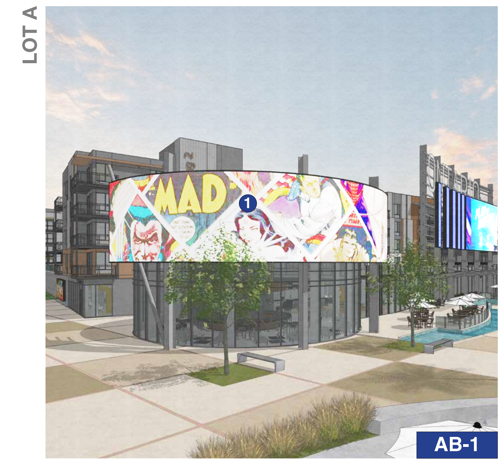
SIZE: 18' H X 96' W X 1'6" D, WRAP AROUND 1/2 THE STRUCTURE HEIGHT OFF GROUND: 18'-0" AREA: 1750 SF ATTACHMENT: FREE STANDING STRUCTURE
