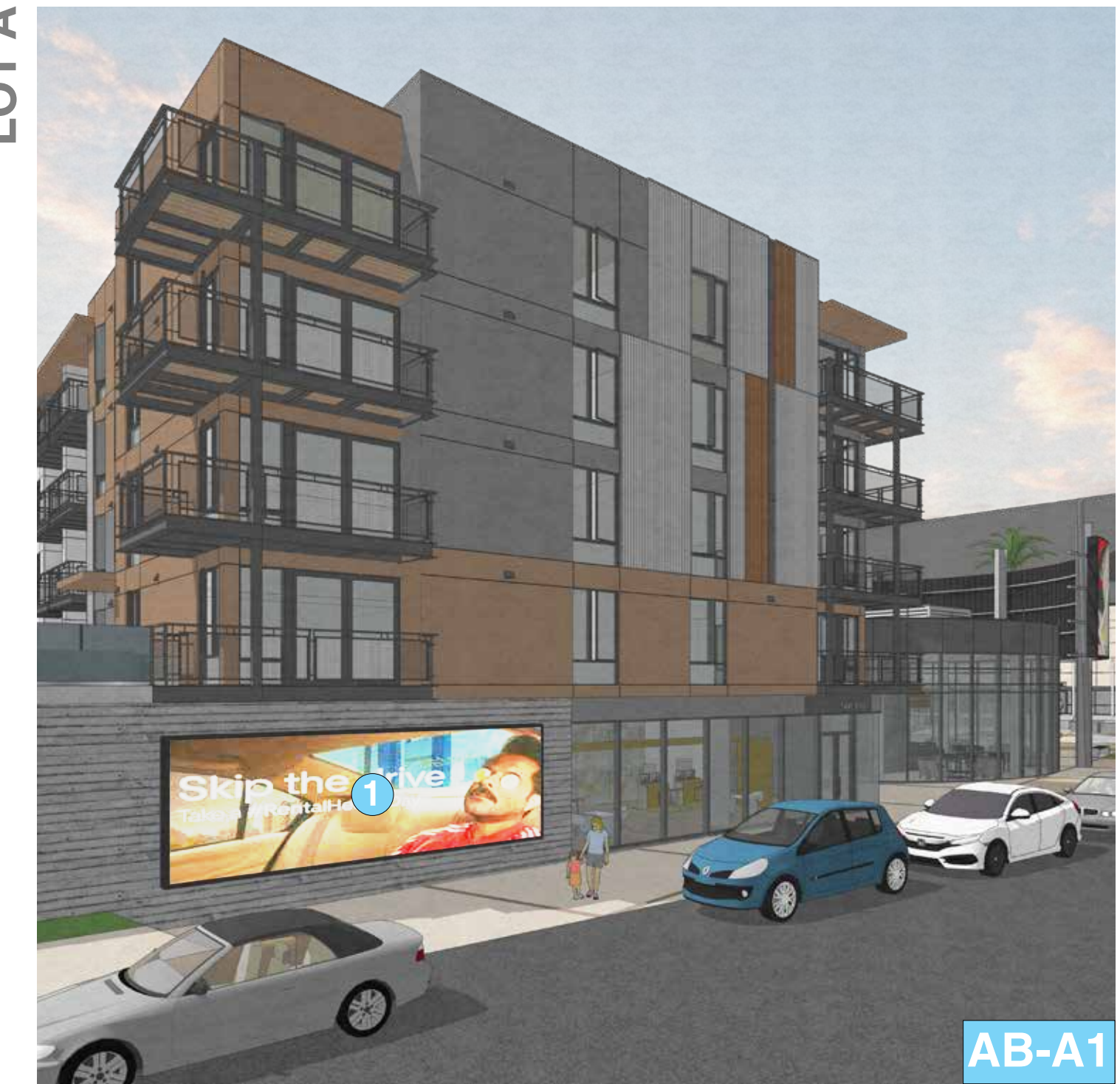
SIZE: 9' H X 27' W X 1'6" D HEIGHT OFF GROUND: 3'-0" AREA: 243 SF ATTACHMENT: WALL MOUNTED TO CONCRETE PARKING GARAGE WALL
