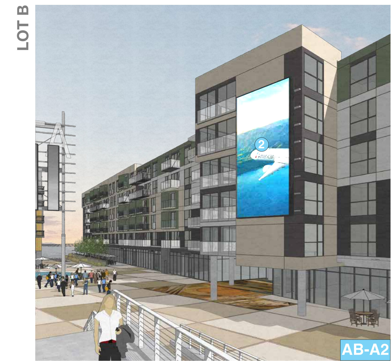
SIZE: 32' H X 18' W X 1'6" D HEIGHT OFF GROUND: 24'-0" AREA: 576 SF ATTACHMENT: WALL MOUNTED TO RESIDENTIAL STRUCTURE
