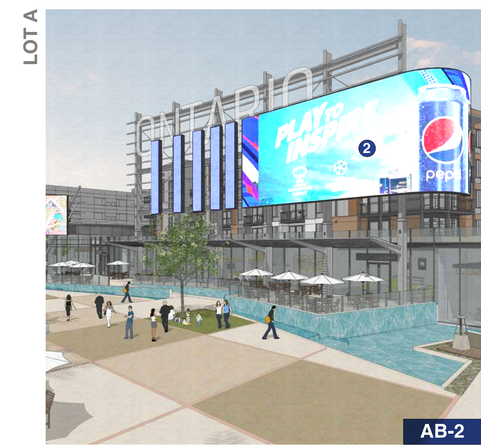
SIZE: LARGE BOARD 27' H X 56' W X 1'6" D, SMALLER BOARDS, 27' H X 4' W X 1'6" D; TYP. HEIGHT OFF GROUND: 25'-0" AREA: 2,410 SF ATTACHMENT: FREE STANDING STRUCTURE
