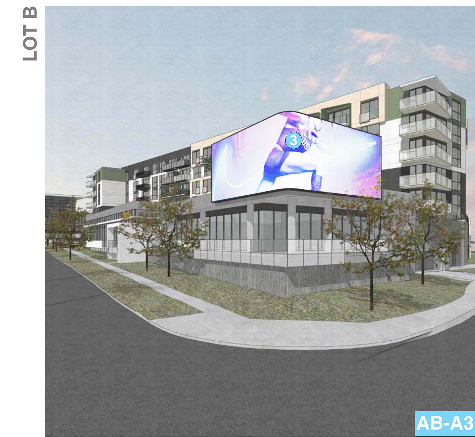
SIZE: 3 BOARDS (18' H X 32' W X 1'6" D) X 2 BOARDS, ADDITIONAL ROUNDED BOARD IN-BETWEEN, 3'8" RADIUS 18' H 5'9" W X 1'6" D HEIGHT OFF GROUND: 25'-0" AREA: 1,255 SF ATTACHMENT: MOUNTED TO CONCRETE STRUCTURE
