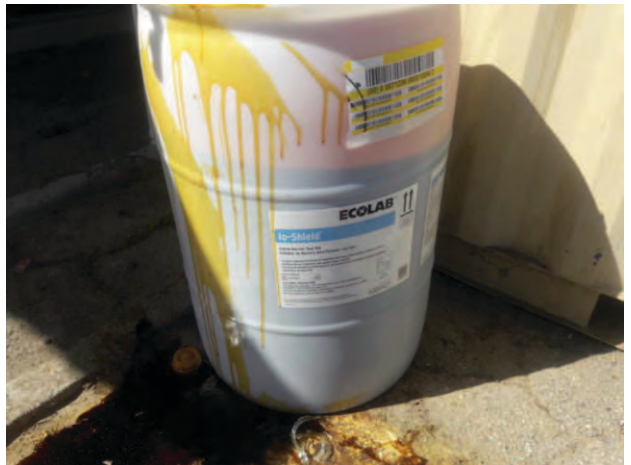
View of 35-gallon drum of iodine and associated leaking.
