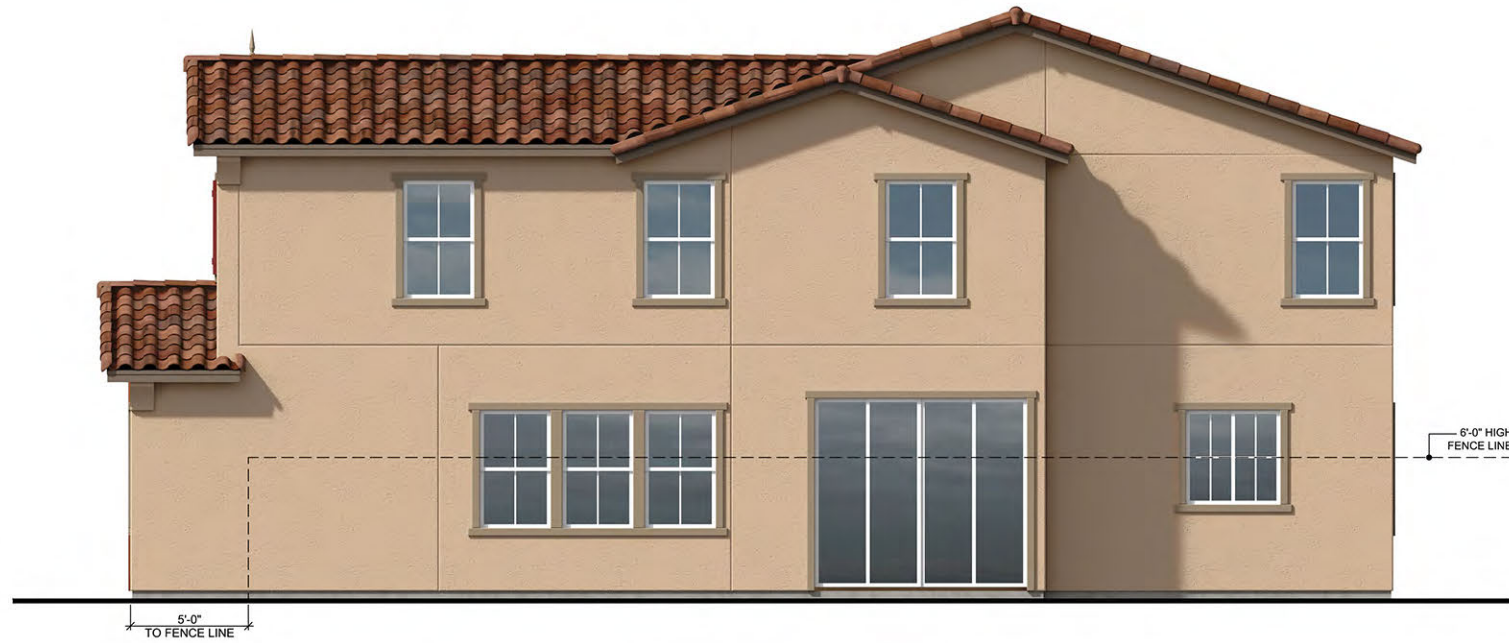
Right Elevation 'A' at Quad Door Option
