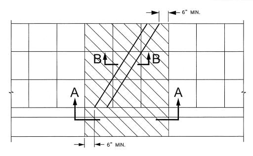
REMOVE AND REPLACE EXISTING CONCRETE. PLACE EXPANSION JOINTS BETWEEN EXISTING AND NEW CONCRETE. ANGLE SHALL BE DETERMINED BY THE INSPECTOR.
