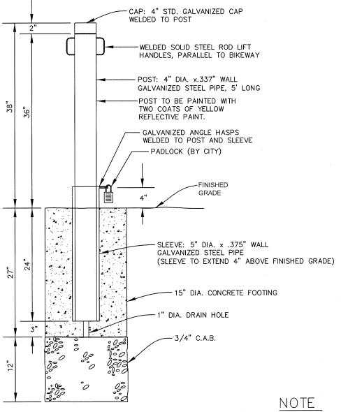
WHEN BOLLARD IS REMOVED FOR MAINTENANCE ACCESS, A TEMPORARY DELINEATOR (E.I. ORANGE CONE) SHALL BE PLACED OVER THE PIPE SLEEVE.
